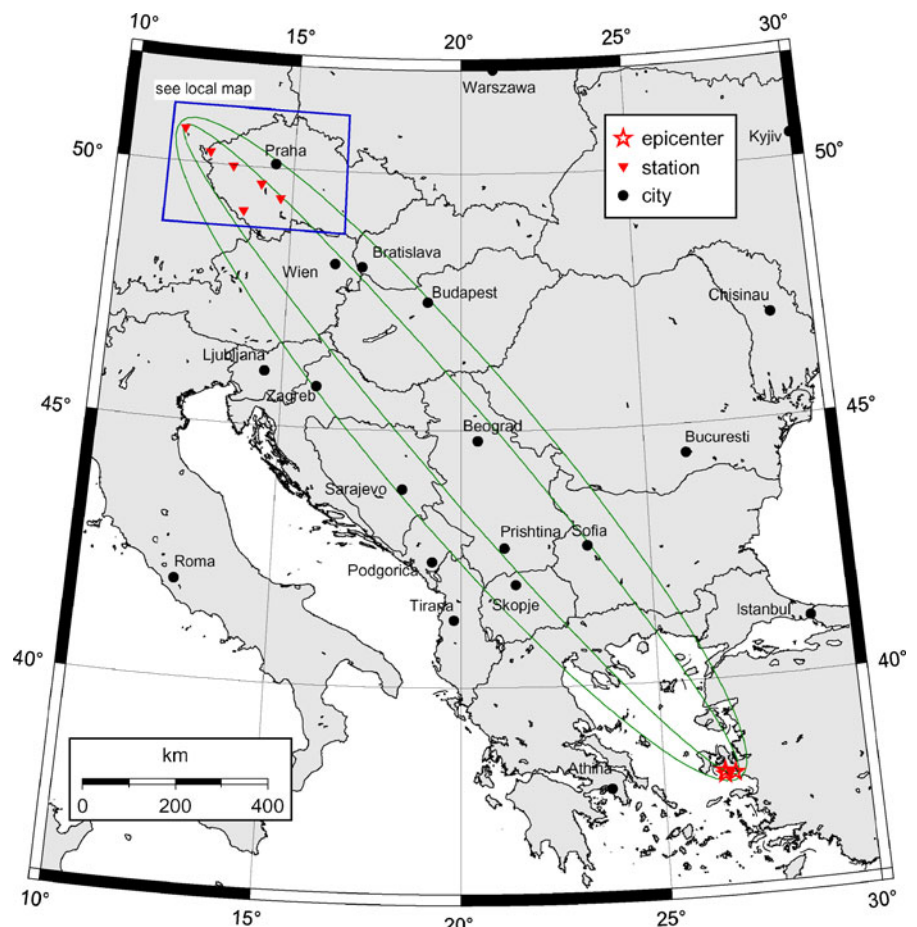
Fig. 1 Surface wave paths across Europe shown in terms of influence zones for 12 and 40 s period surface waves. The epicenters of three Aegean Sea earthquakes are situated close to one another
